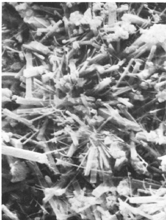
Fig. 17. Macro-crystal forms of aluminosilicate on the surface of support after gas washing (SEM, 5940 \times ).
