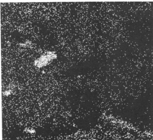
Fig. 7. Distribution of alumina in supports after gas washing: facial distribution.
